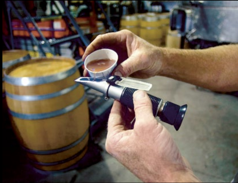
Freshly picked grapes are squeezed for their sugar content in a sugar refractometer. The brix, or sugar content, measured lets the winemaker know if it's time to harvest the grapes.
